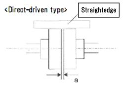
Make an adjustment with a straightedge so that the outer edges of the shaft couplings on the right and left can align with each other and clearance (a) can be uniform over the entire circumference.
